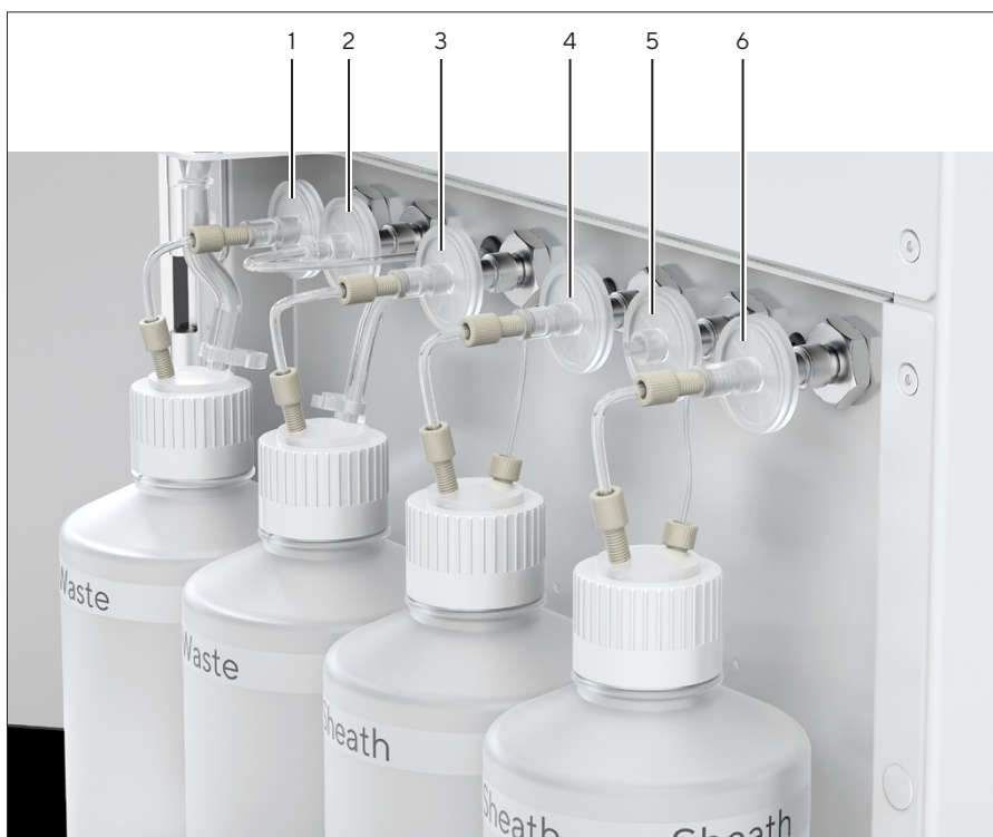
Fig. 5: Filters, fluid bay
