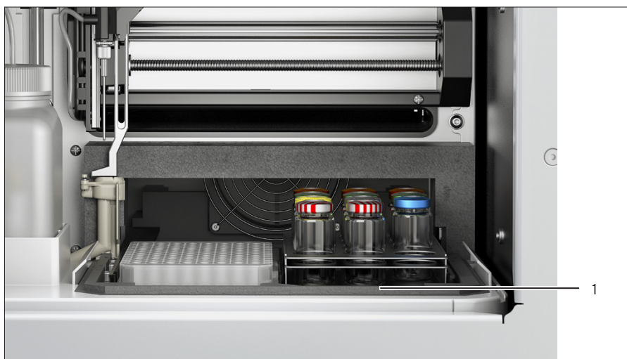
Fig.16: Inserted sample plate and consumables vial rack
